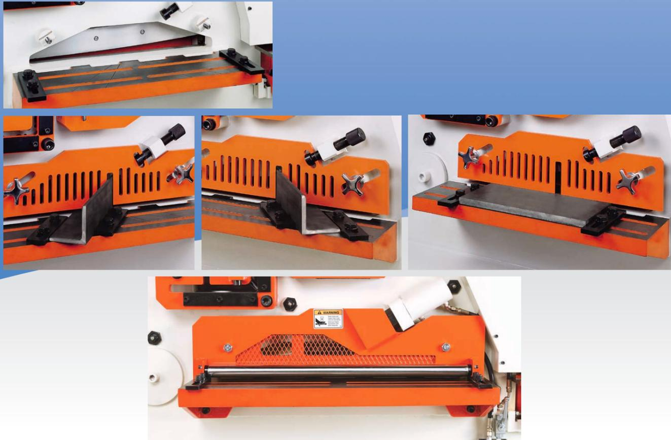
\*Optional hydraulic hold-down for double cylinder ironworkers. (Standard on IW-165SD)
